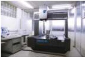
Measuring a housing on a 3D measuring machine
